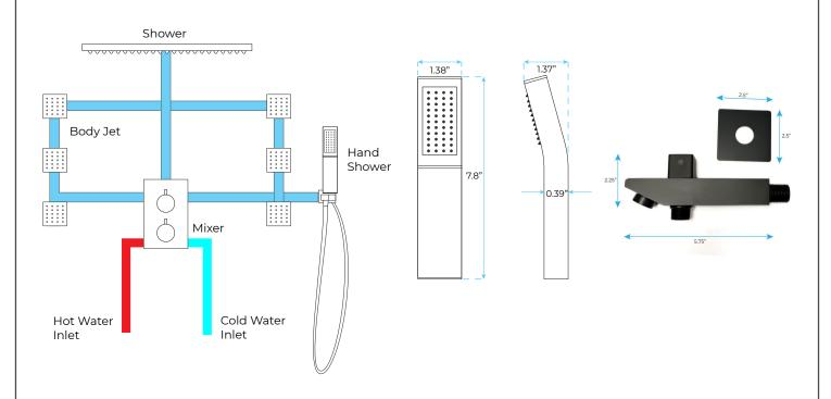
The minimum required water pressure is 0.05 MPa (0.5 bar).
